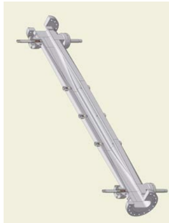
Fig. 27: Mechanical drawing of the kicker.
